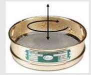
Vertical vibration is generated by the on/off frequency of the electromagnetic drive. However, vertical vibration is not enough to impart the correct movement for sieving. The shaker also needs to twist the sieve stack - this rotating action ensures the sample passes over the full surface of the sieve and the maximum number of apertures to give rapid accurate results
