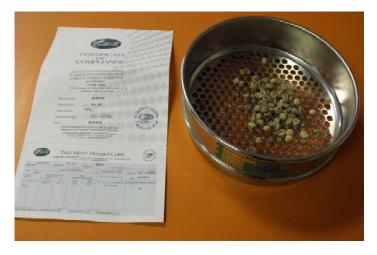
Coffee Laboratory Machine Grading Screens are made from sturdy stainless steel frames, suitable for use on a laboratory sieve shaker. Manufactured and certified in compiance with ISO 3310 Specification for perforated steel plate sieves.
