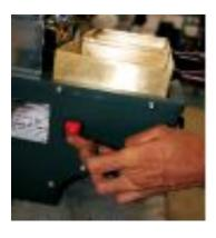
**1.** Switch on the main switch of the roaster. Check to ensure that the roasting drum is rotating counterclockwise.
