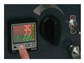
**4.** Set the temperature to the desired temperature by pressing up "S" or down "T" (we recommend 220-230°C). The gas supply will automatically be turned off depending on the actual temperature inside the drums (in accordance to set temperature).
