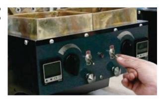
**3.** Turn up the gas-adjusting knob to obtain a blue flame and even fire.
