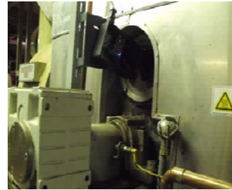
THE LASER MODULE CAN BE MOUNTED AT THE VIEWING WINDOW FOR REAL TIME COLOR MONITORING, OR OVER THE HOPPER, AFTER COOLING, FOR FINISHED PRODUCT COLOR ANALYSIS, AND LOGGING
