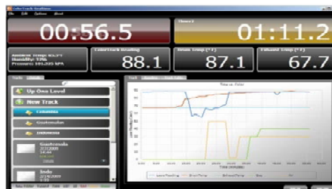
COLORTRACK ROASTLOG SOFTWARE DISPLAYS ALL DATA IN REAL TIME. DATA IS AUTOMATICALLY LOGGED, AND CAN BE EXPORTED AND SAVED TO EXCEL FORMAT.
