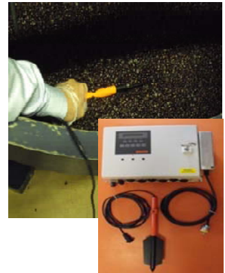
SINAR DRYPRO INLINE MOISTURE CONTROL BOX AND SENSOR . SENSOR READS TOTAL MOISTURE, IN HOPPER AFTER COOLING.
