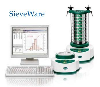
SieveWare, the software for particle size analyses, exceeds manual evaluation in many aspects, due to the fact that the software is able to automatically control the necessary measurement and weighing procedures – from the registration of the weight of the sieve up to the evaluation of the data.
