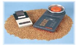
THE SINAR AP 6060 MOISTURE MSRP \$3,295.00 **ANALAYZER IS USED BY OVER 60%** OF THE COFFEE INDUSTRY TO **MEASURE MOISTURE, AND DENSITY IN ALL FORMS OF COFFEE.**
