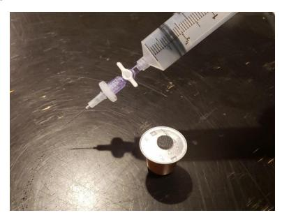
Remove the needle and attach the small plastic "double connector".
