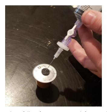
NOTE: Pull slowly and carefully. If you use too much force, and spring a leak in the package, the plunger will be suddenly easier to pull.
