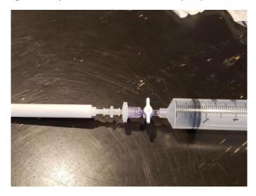
Turn the valve to the open position. (The closed position is pictured above)
