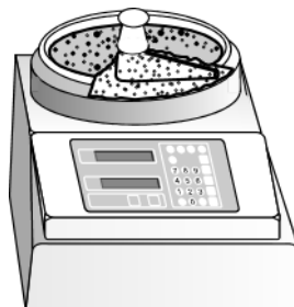
Air Jet Sieve (for sieves 20 - 1000µm)
