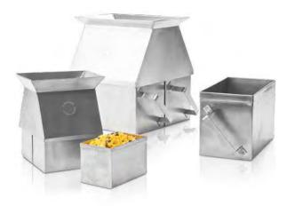
These hand held sample dividers will subdivide material samples into two smaller portions by a single pass or further subdivisions can be attained by multiple passes. The important feature of Endecotts sample dividers is that each subdivision retains the characteristics of the original sample. Based on the recommendations of BS 5309 and BS 3406/1. Produced in stainless steel with slot widths of either 6.35 mm ( $\frac{1}{4}$ ") or 12.7 mm ( $\frac{1}{2}$ ").
