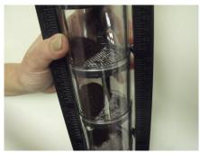
Gradations on the side of the holder, are marked 0 to 100 for each section.
