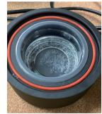
How to make a saturated brine: There is an empty bottle in the AW-600 hard case, you will see there are 2 lines marked "WATER" and "NaCl" on the bottle. Put NaCl (Salt) in the bottle till the amount reaches the line of "NaCl", then pour tape water or distilled water in the bottle till reaches the line of "WATER", close the lid and shake it to mix the water and NaCl and leave it at least 8 hours, then use the brine for calibration. The brine can be recycled for next time using
