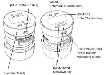
Press the System Reset button by paperclip or pen point to reset system in case the system is crashed
