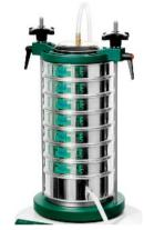
The O-ring seals are fitted on to the outside of the bottom rim of each sieve, which means the sieves are stacked onto each other and they form a seal.
