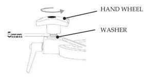
Place the two large plain washers over the 20mm threads of the clamp sleeves. These can be seen protruding vertically from the two side lugs on the clamp plate. Screw the two hand wheels loosely onto the 20mm threads; leave a gap of 5 mm between the large washer and the hand wheel face. Do not tighten right down at this point.
