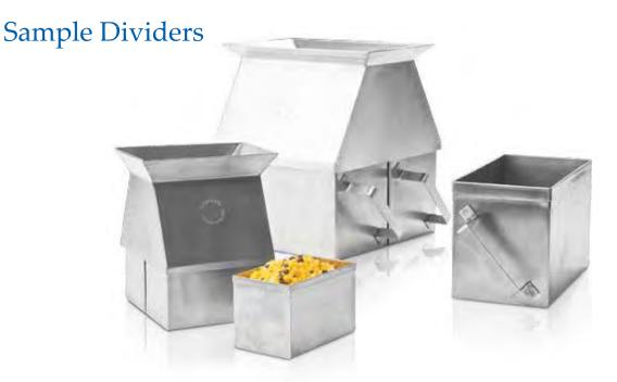
These hand held sample dividers will subdivide material samples into two smaller portions by a single pass or further subdivisions can be attained by multiple passes. The important feature of Endecotts sample dividers is that each subdivision retains the characteristics of the original sample. Based on the recommendations of BS 5309 and BS 3406/1. Produced in stainless steel with slot widths of either 6.35 mm (1/4") or 12.7 mm (1/2").
