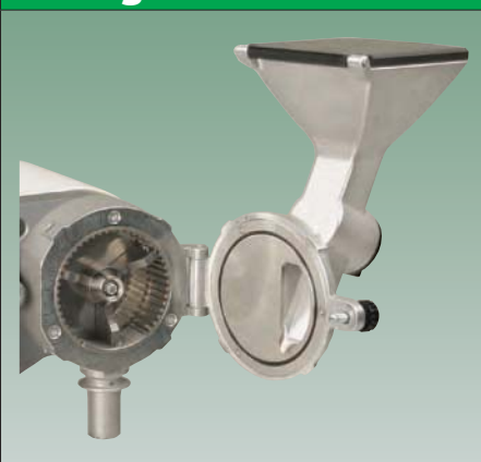
Milling chamber with Safety switch, funnel, lid, rotary slide for product dosage and NS29 adapter for intercepting tubes
