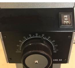
Main Switch is a 3-way switch with Off, ON and Run positions
