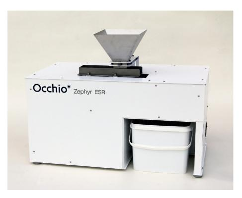
Instrument : Zephyr ESR C Resolution: from 5 to 50  $\mu m/pixel$  depending on the optical configuration. Measurement time: less than 5 minutes
