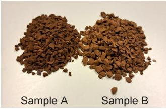
The disparity between the two samples can be easily observed in the image depicted below. Thanks to the capabilities of the Armadillo software and the Zephyr ESR C instrument, this difference can be measured and quantified accurately during particle size measurement in QC.
