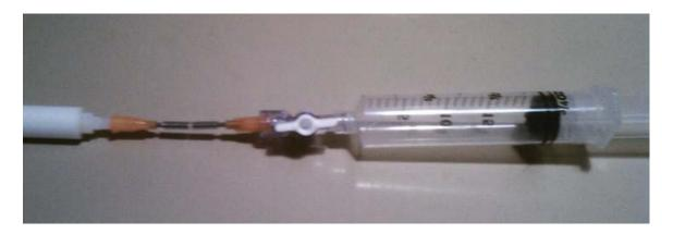
Turn the on-off valve to the open position (as pictured above) and gently depress the plunger to inject the syringe contents into the sensor. As the plunger is depressed, the O2 reading will decrease to the value in the package/bottle. Leave the syringe connected and the reading will reach its equilibrium point.
