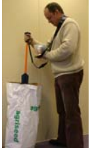
The SINAR SP 6600 is designed for insertion in to bulk food stuffs, like this bag of grain.
