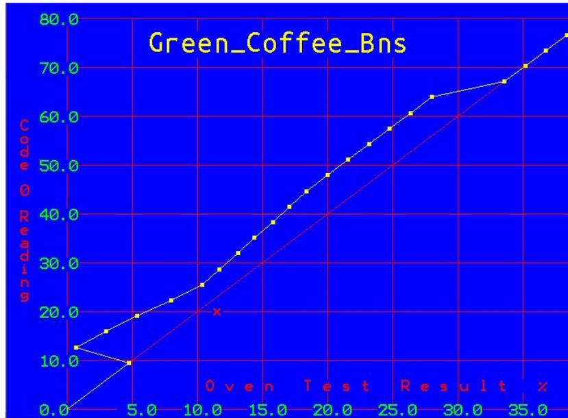
To use a sample of green coffee to calibrate a Sinar Moisture Analyzer
